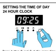
Press button B and C at the same time and while turning knob A enter the time of day.
